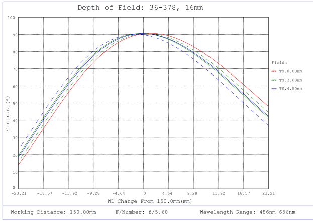
#36-378, 16mm FL f/5.6 Rugged Blue Series M12 Lens, Depth of Field Plot, 150mm Working Distance, f5.6
