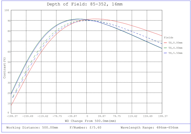
#85-352, 16mm, f/5.6 Ci Series Fixed Focal Length Lens, Depth of Field Plot, 500mm Working Distance, f5.6
