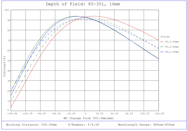
#85-351, 16mm, f/4 Ci Series Fixed Focal Length Lens, Depth of Field Plot, 500mm Working Distance, f4
