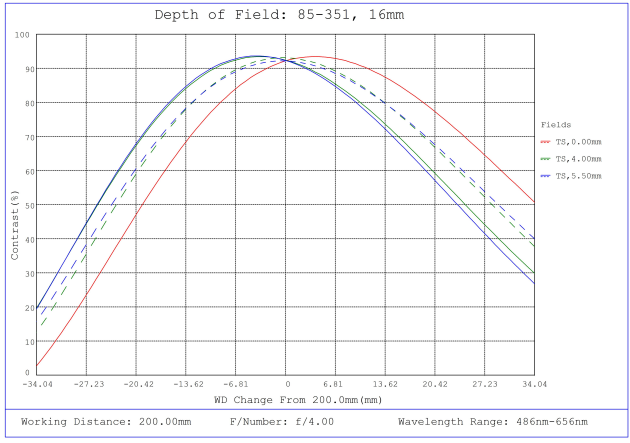
#85-351, 16mm, f/4 Ci Series Fixed Focal Length Lens, Depth of Field Plot, 200mm Working Distance, f4
