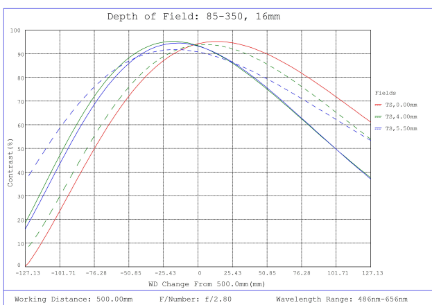
#85-350, 16mm, f/2.8 Ci Series Fixed Focal Length Lens, Depth of Field Plot, 500mm Working Distance, f2.8
