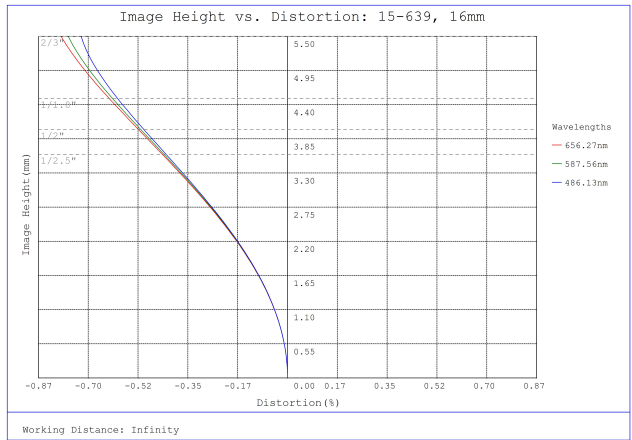
#15-639, 16mm, f/1.8 Cw Series Fixed Focal Length Lens, Distortion Plot
