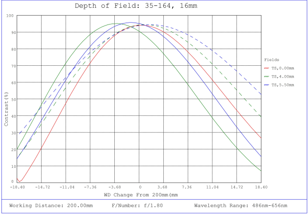
#35-164, 16mm, f/1.8 Cr Series Fixed Focal Length Lens, Depth of Field Plot, 200mm Working Distance, f1.8
