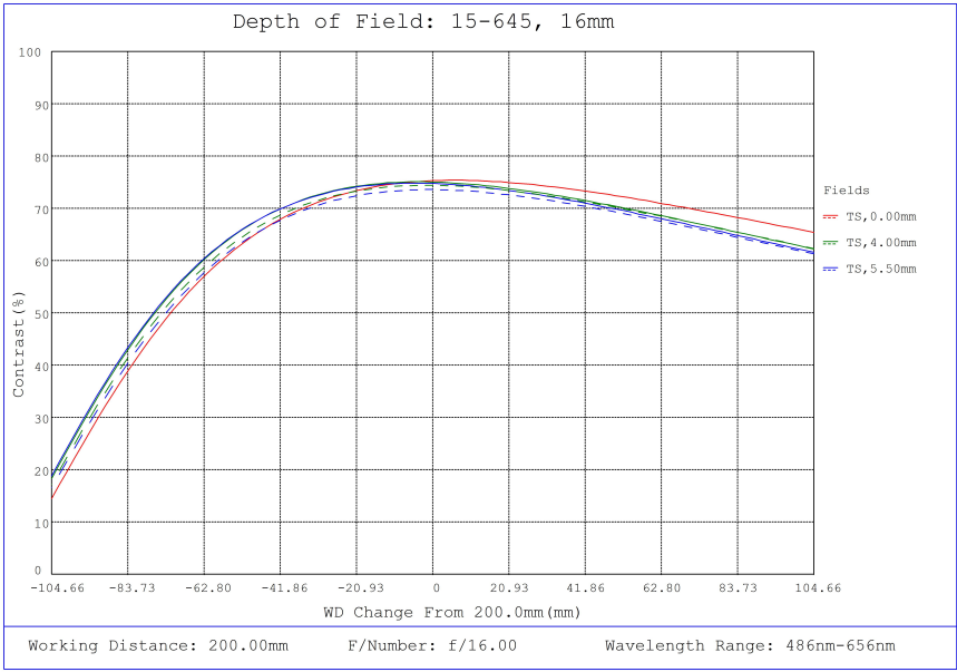
#15-645, 16mm, f/16 Cw Series Fixed Focal Length Lens, Depth of Field Plot, 200mm Working Distance, f16
