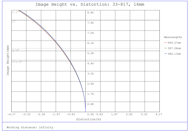
#33-817, 16mm f/5.6, HPI Series Fixed Focal Length Lens, Distortion Plot
