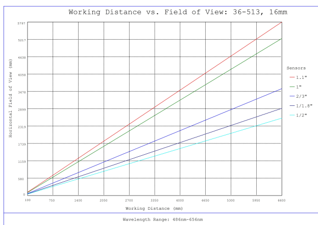
#36-513, 16mm f/4, HPr Series Fixed Focal Length Lens, Working Distance versus Field of View Plot
