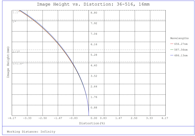
#36-516, 16mm f/11, HPr Series Fixed Focal Length Lens, Distortion Plot
