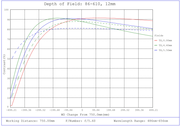
#86-610, 12mm, f/5.6 Ci Series Fixed Focal Length Lens, Depth of Field Plot, 750mm Working Distance, f5.6
