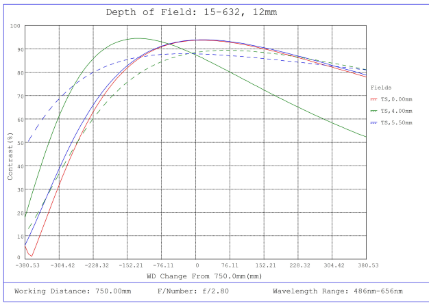
#15-632, 12mm, f/2.8 Cw Series Fixed Focal Length Lens, Depth of Field Plot, 750mm Working Distance, f2.8
