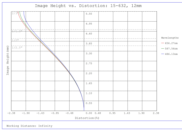
#15-632, 12mm, f/2.8 Cw Series Fixed Focal Length Lens, Distortion Plot
