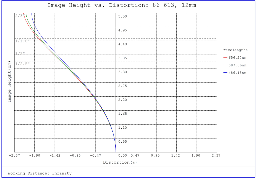
#86-613, 12mm, f/16 Ci Series Fixed Focal Length Lens, Distortion Plot
