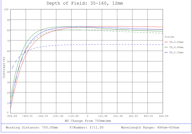
#35-160, 12mm, f/11 Cr Series Fixed Focal Length Lens, Depth of Field Plot, 750mm Working Distance, f11
