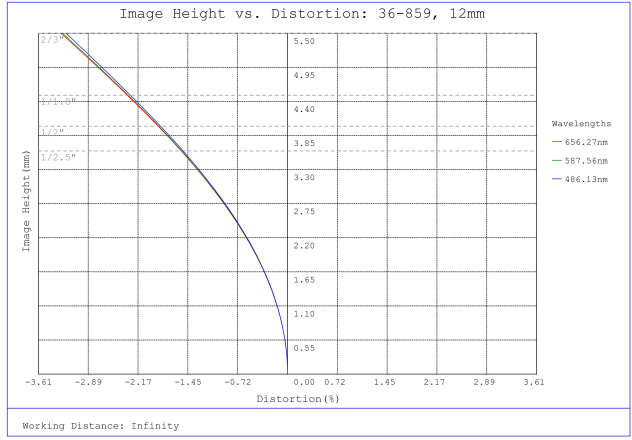
#36-859, 12mm f/8, 400-2000mm Primary WD, HRr Series Fixed Focal Length Lens, Distortion Plot
