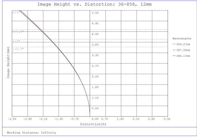
#36-858, 12mm f/8, 150-500mm Primary WD, HRr Series Fixed Focal Length Lens, Distortion Plot
