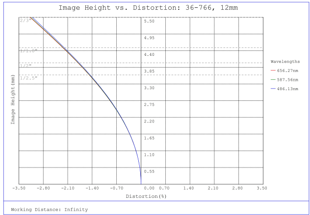
#36-766, 12mm f/8, 150-500mm Primary WD, HRi Series Fixed Focal Length Lens, Distortion Plot
