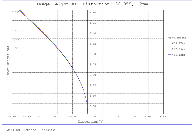
#36-855, 12mm f/5.6, 150-500mm Primary WD, HRr Series Fixed Focal Length Lens, Distortion Plot
