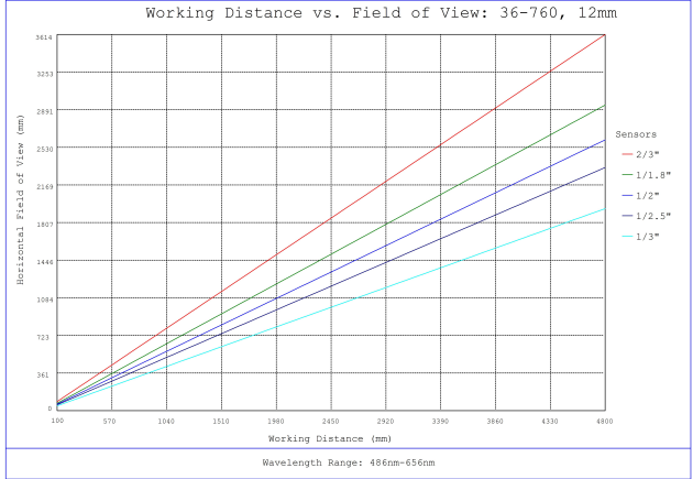
#36-760, 12mm f/4, 150-500mm Primary WD, HRi Series Fixed Focal Length Lens, Working Distance versus Field of View Plot
