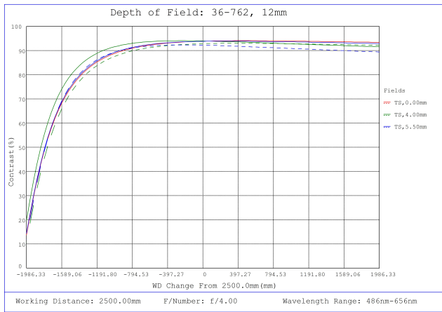
#36-762, 12mm f/4, 1000mm-∞ Primary WD, HRI Series Fixed Focal Length Lens, Depth of Field Plot, 2500mm Working Distance, f4
