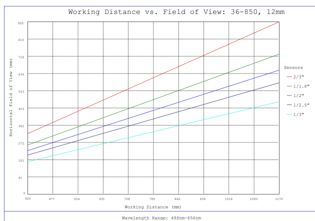
#36-850, 12mm f/2.8, 400-2000mm Primary WD, HRr Series Fixed Focal Length Lens, Working Distance versus Field of View Plot
