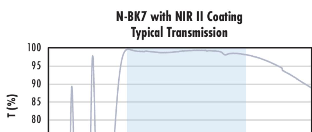
Typical transmission of a 3mm thick N-BK7 window with NIR II (750 - 1550nm) coating at 0° AOI.
