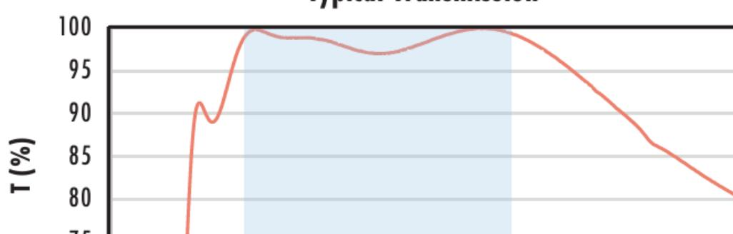
Typical transmission of a 3mm thick N-BK7 window with YAG-BBAR (500-1100nm) coating at 0° AOI.
