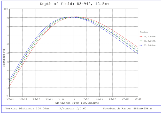
#83-942, 12.5mm FL f/5.6, Blue Series M12 Lens, Depth of Field Plot, 150mm Working Distance, f5.6
