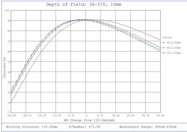
#36-370, 10mm FL f/5.6, Rugged Blue Series M12 Lens, Depth of Field Plot, 150mm Working Distance, f5.6
