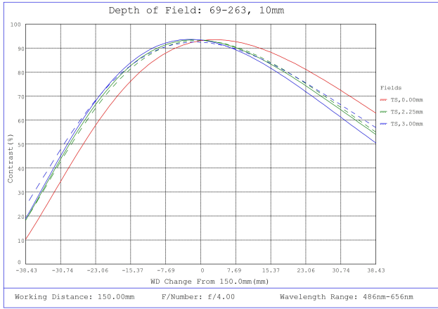
#69-263, 10mm FL f/4, Blue Series M12 Lens, Depth of Field Plot, 150mm Working Distance, f4
