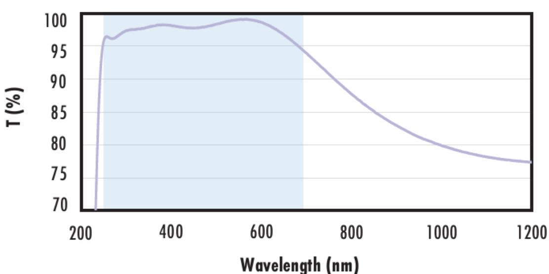
Typical transmission of a 3mm thick fused silica window with UV-VIS (250-700nm) coating at 0° AOI.
