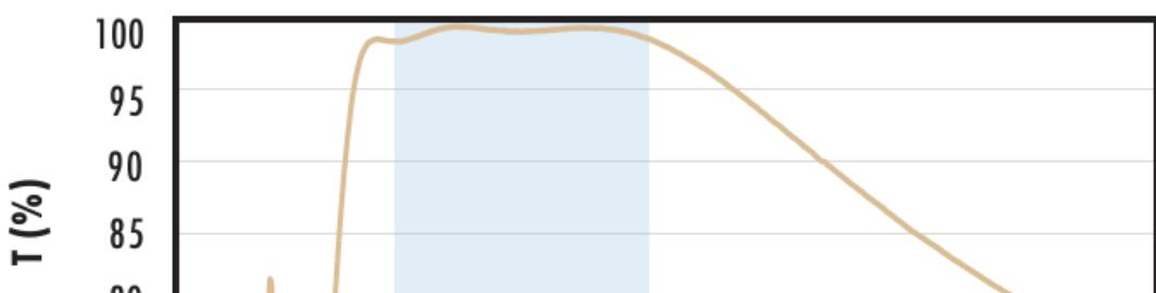
Typical transmission of a 3mm thick fused silica window with VIS (425-675nm) coating at 0° AOI.
