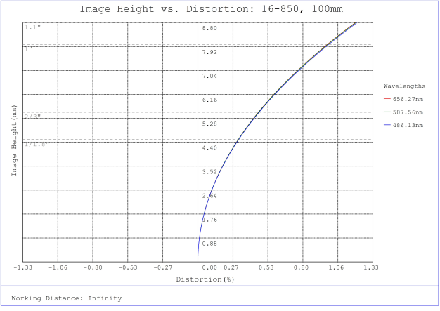
#16-850, 100mm, f/5.6 Athermal Lens, Distortion Plot
