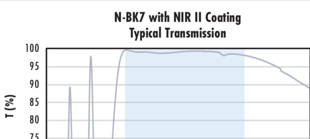
Typical transmission of a 3mm thick N-BK7 window with NIR II (750 - 1550nm) coating at 0° AOI.
