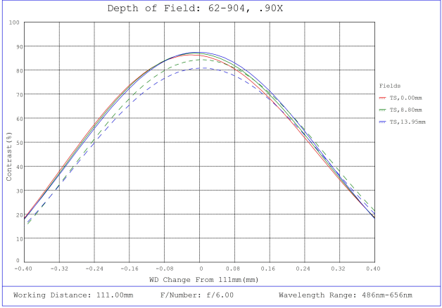
#62-904, 0.9X, 28.7mm M42 x 1.0 (19.53mm) PlatinumTL™ Telecentric Lens, Modulated Transfer Function (MTF) Plot, 111mm Working Distance, f6
