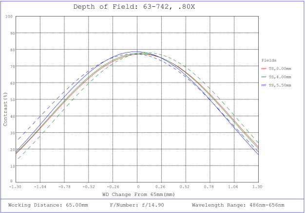
#63-742, 0.8X, 65mm WD CompactTL™ Telecentric Lens, Depth of Field Plot, 65mm Working Distance, f14.9
