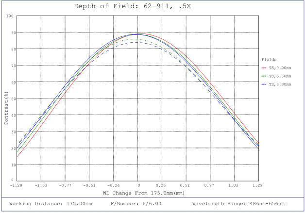
#62-911, 0.5X CobaltTL Telecentric Lens, Depth of Field Plot, 175mm Working Distance, f6
