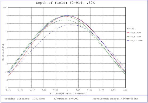
#62-914, 0.5X, 28.7mm M42 x 1.0 (19.53mm) PlatinumTL™ Telecentric Lens, Modulated Transfer Function (MTF) Plot, 175mm Working Distance, f6
