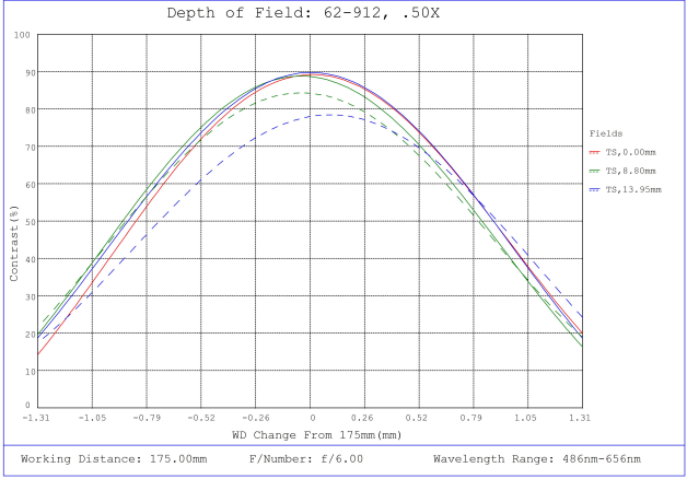
#62-912, 0.5X, 28.7mm F-Mount PlatinumTL™ Telecentric Lens, Modulated Transfer Function (MTF) Plot, 175mm Working Distance, f6
