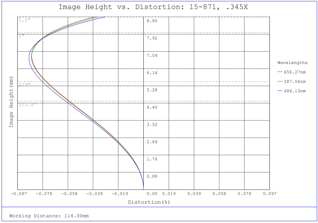
#15-871, 0.345X In-Line CobaltTL Telecentric Lens, Distortion Plot
