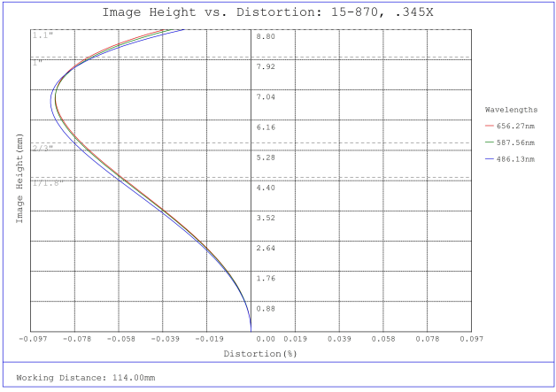
#15-870, 0.345X CobaltTL Telecentric Lens, Distortion Plot
