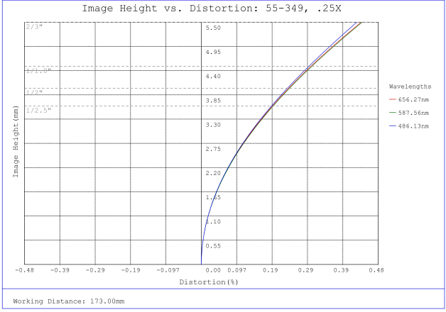
#55-349, 0.25X 2/3" GoldTL™ Telecentric Lens, Distortion Plot
