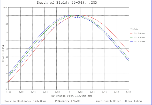
#55-349, 0.25X 2/3" GoldTL™ Telecentric Lens, Depth of Field Plot, 173mm Working Distance, f6
