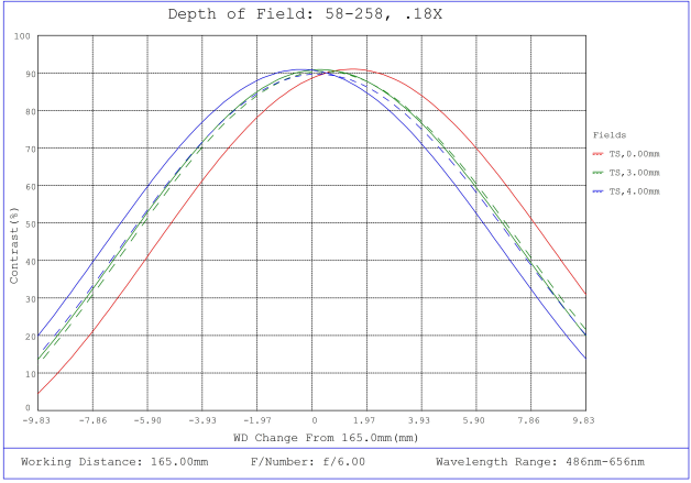
#58-258, 0.18X ½" GoldTL™ Telecentric Lens, Depth of Field Plot, 165mm Working Distance, f6
