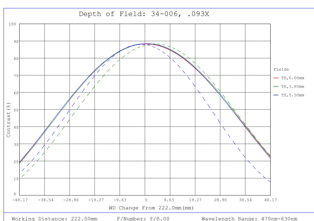
#34-006, 0.093X, 2/3" C-Mount TitanTL® Telecentric Lens, Depth of Field Plot, 222mm Working Distance, f8
