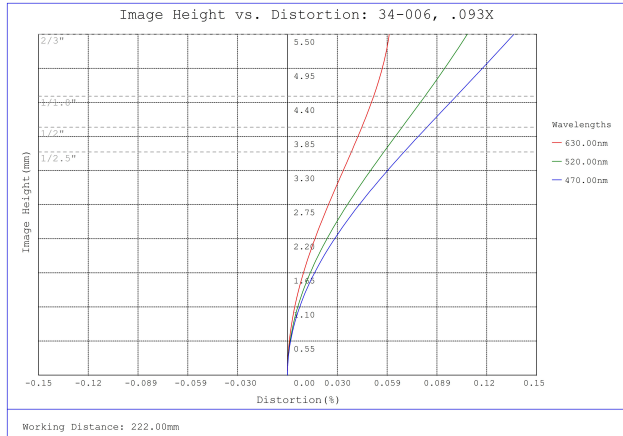
#34-006, 0.093X, 2/3" C-Mount TitanTL® Telecentric Lens, Distortion Plot
