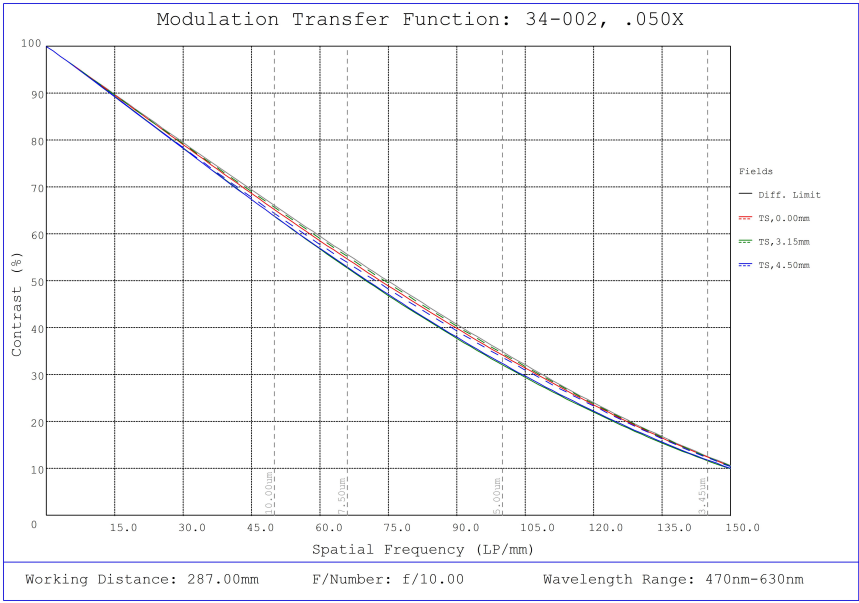
#34-002, 0.050X, 1/1.8" C-Mount TitanTL® Telecentric Lens, Modulated Transfer Function (MTF) Plot, 287mm Working Distance, f10
