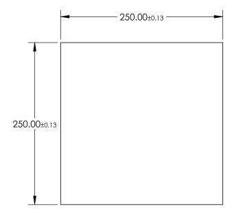
SPECIFICATIONS SUBJECT TO CHANGE WITHOUT NOTICE PARTS TO THIS DRAWING DIMENSIONS ARE FOR REFERENCE ONLY **S**2 **Edmund Optics®** S1 **PLANO PLANO** SHAPE 80-50 80-50 SURFACE QUALITY 250 x 250mm Uncoated, Gorilla Glass® THIRD ANGLE PROJECTION 225.0 x 225.0 225.0 x 225.0 TITLE CLEAR APERTURE Window N/A N/A COATING APERTURE SHEET DWG NO ALL DIMS IN PROTECTIVE AS NEEDED PROTECTIVE AS NEEDED 17161 **BEVEL** 1 OF 1
