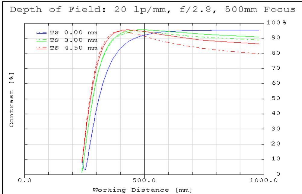
**Figure 8:** Polychromatic diffraction through-focus MTF at 20 linepairs/mm (image space). Contrast is plotted to two times the focus distance. Note object spatial frequency changes with working distance.
