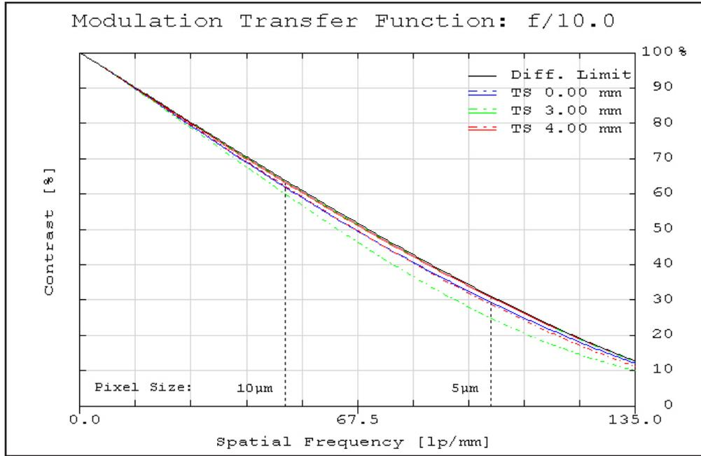
**Figure 5:** Image space polychromatic diffraction FFT Modulation Transfer Function (MTF) for  $\lambda = 486\text{nm}$  to  $656\text{nm}$ . Included are Tangential and Sagittal values for field points on center, at 70% of full field and at the maximum sensor format. Solid black line indicates diffraction limit determined by  $f/\#$ -defined aperture. Frequencies corresponding to the Nyquist resolution limit of pixel sizes are indicated.
