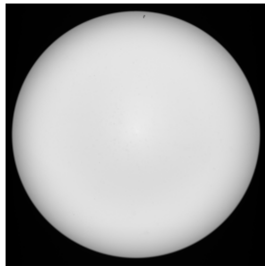
Figure 6: Real-world test result for the new design, showing a more even irradiance profile than the original design
